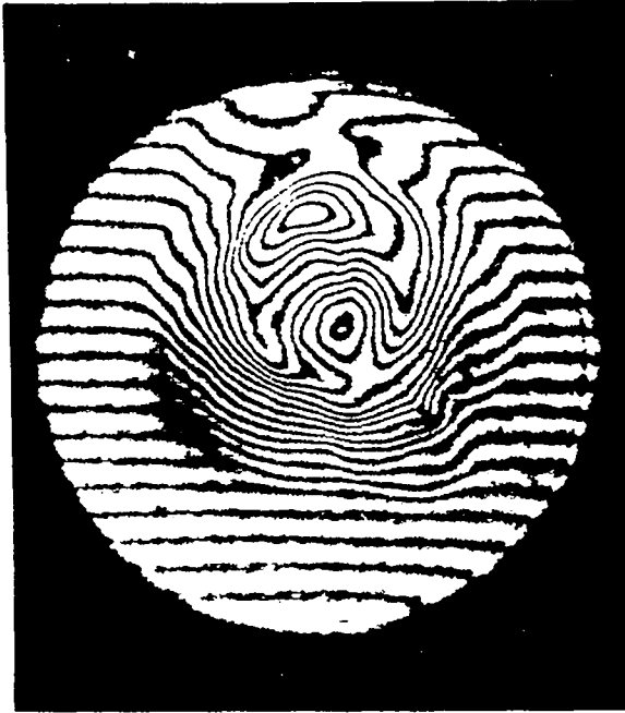
Fig. 7. End-on interferogram of Scylla IV-3 with \ell = 1 field over the 3-meter length.
